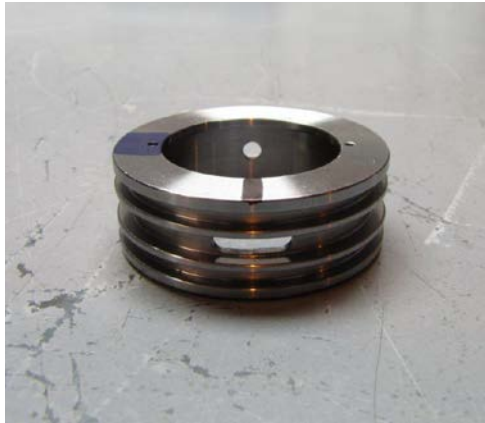
(9) Mark the sleeve above the slot If you are going to use any type of locking substance, apply it to the case
