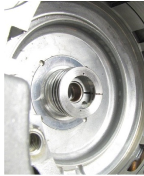
(8) The slot in the case feeds the sleeve case and sleeve slots must be aligned
