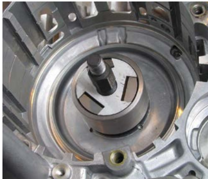
(3) Remove the sleeve from the case with the appropriate puller, you can heat the sleeve before removing
