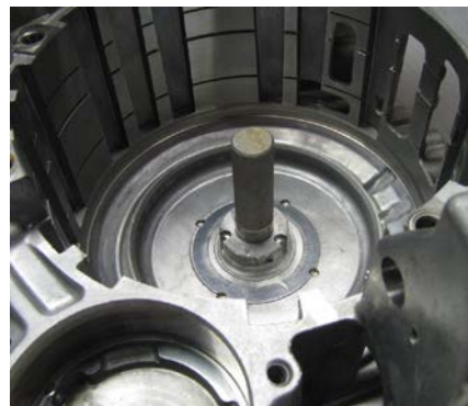
(6) Use bushing driver to properly install new bushing
