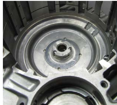
(4) Now might be a good time to replace the bushing
