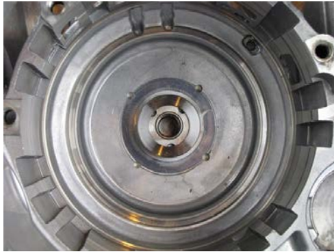
(1) The TF-60SN K2 clutch sealing ring sleeve can rotate and cause clutch failure
